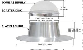
DOME ASSEMBLY: DOME SEALED WITH HIGH PERFORMANCE SEALANT AND LOCKED ONTO AN ALUMINUM RING TO ELIMINATE ANY STRESS AND INCREASE LONG TERM DURABILITY. UNIQUE DESIGN TO ALLOW ANY CONDENSATION BUILD-UP TO ESCAPE BY SITTING OUTSIDE THE FLASHING.
