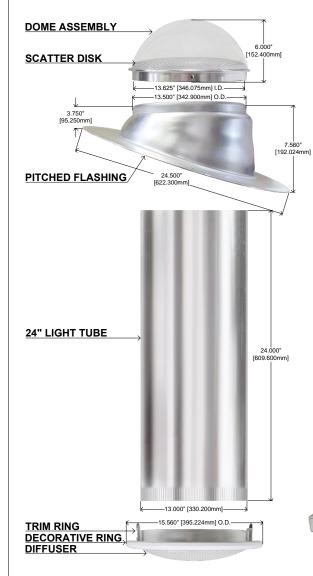
DOME ASSEMBLY: DOME SEALED WITH HIGH PERFORMANCE SEALANT AND LOCKED ONTO AN ALUMINUM RING TO ELIMINATE ANY STRESS AND INCREASE LONG TERM DURABILITY. UNIQUE DESIGN TO ALLOW ANY CONDENSATION BUILD-UP TO ESCAPE BY SITTING OUTSIDE THE FLASHING.
