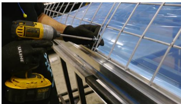
Install Screen Connector Clips
