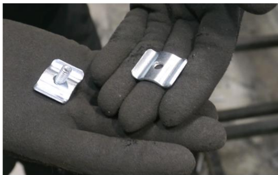
Dis-assemble Screen Connector Clips
